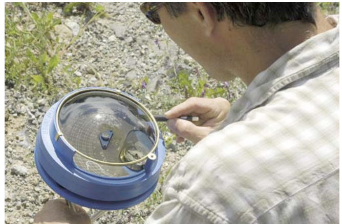
Using a white grease pencil to trace the horizon line under the Solar Pathfinder's reflective dome.
